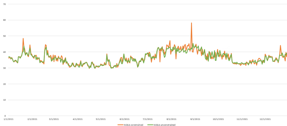
Figure 4: Comparison of the average daily historical constrained and unconstrained market clearing prices [$/MWh]
